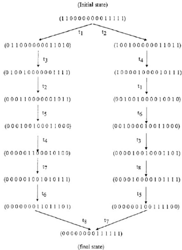
FIGURE 8.4 A partial portion of the reachability graph for the Petri net model shown in Figure 8.3.
